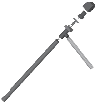
Diagram 3. Design of pellet auger
